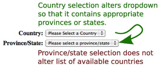
Figure 6.1: An partial address form demonstrating a non-symmetric use of page-channels.
