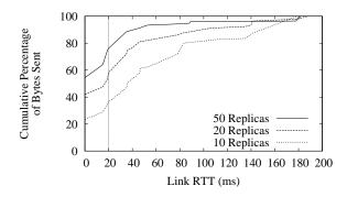
Figure 7: *Results of the Stream Benchmark.* The graph shows the percentage of bytes sent over links of different latency as the number of replicas varies.
