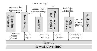
Figure 3: *Prototype Software Architecture*. Pond is built atop SEDA. Components within a single host are implemented as *stages* (shown as boxes) which communicate through events (shown as arrows). Not all stages run on every host; only inner ring hosts run the Byzantine agreement stage, for example.
