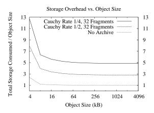
Figure 4: *Storage Overhead.* Objects of size less than the block size of 8 kB still require one block of storage. For sufficiently large objects, the metadata is negligible. The cost added by the archive is a function of the encoding rate. For example, a rate 1/4 code increases the storage cost by a factor of 4.8.
